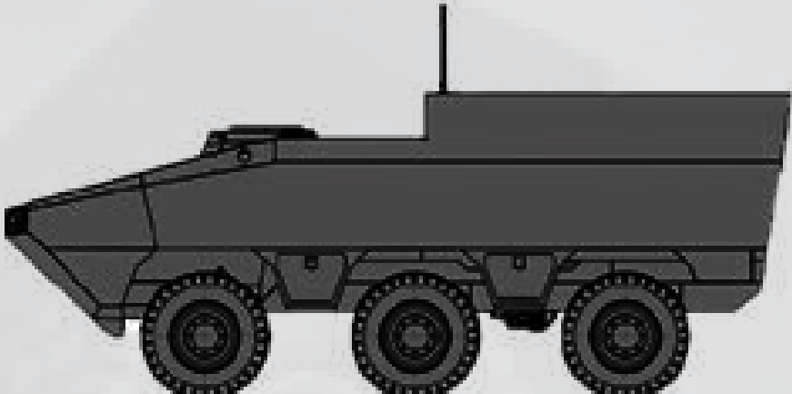
With heightened hull (for C2/ medivac)
